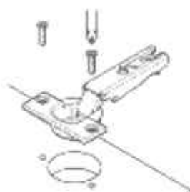
Cup for screw fixing: Preferably with countersunk chipboard screws
