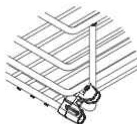
2. Insert Clip-2 to back end of basket & rotate to fix it
